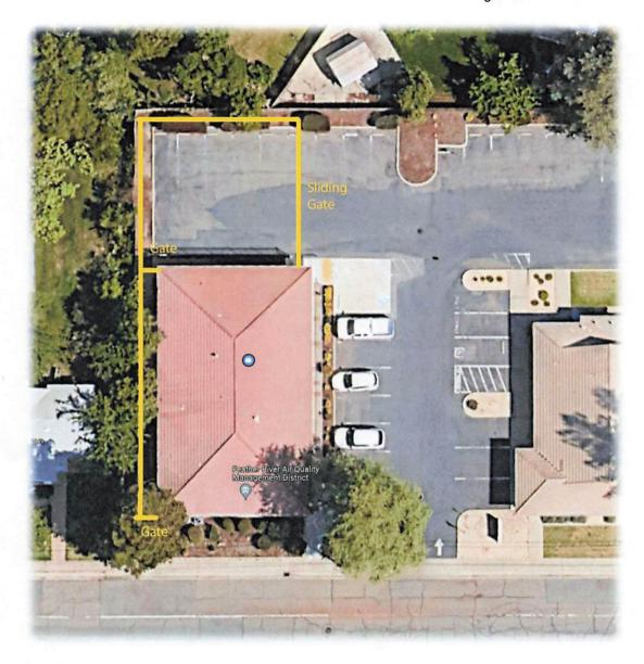
In addition to the fence three gates would be required, one facing the street, one facing the rear parking area and one sliding gate to allow vehicle access. All gates will be equipped with the required emergency hardware.
